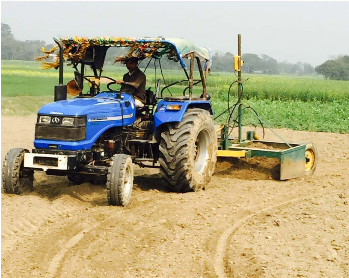
Figure 14. Smallholder use of laser land leveler in rice/wheat rotations in Eastern India.
